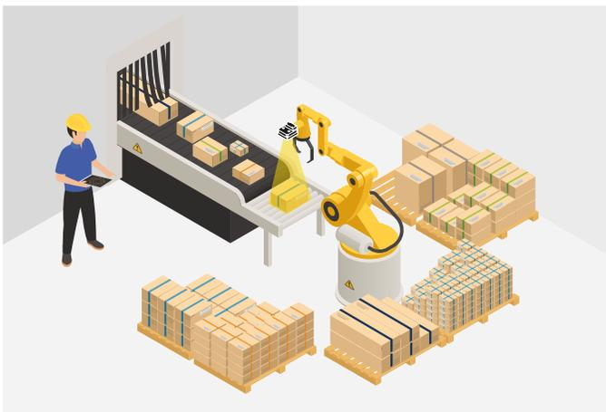
Next day delivery and mixed pallets require fast and versatile robots to stake any article tightly onto a pallet. Therefore, machine vision is required to guide the robot. The camera data is used to determine the shape, position and orientation of the pickable object and to find its best lifting point. Robustness, compact size and light weight allow its assembly on the robot arm.
