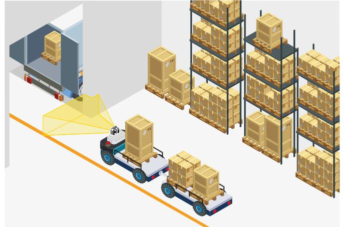
Navigation, obstacle detection, docking and pick-up require a complete and detailed overview of the environment. The blaze camera captures the entire scene in real-time, at daylight or in darkness. Its compact and robust design facilitates an easy integration. The built-in, powerful processor minimizes the CPU load on the vehicle's embedded controller.
