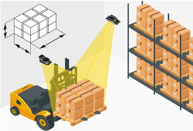
To plan and optimize the space and costs in a warehouse or transport vehicle, it is essential to know the weight but also the exact size of the pallets and parcels. The Basler blaze camera is ideal for size measurement tasks. Its precision, speed, robustness, compact size and Gigabit Ethernet interface are suitable for accurate, flexible, on-the-fly measurements wherever needed in your facility. If color is needed as well, you can combine and synchronize it with any of Basler's 2D cameras.
