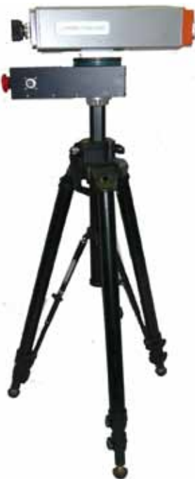
Spectral Camera PS mounted on a rotary stage on top of a tripod
