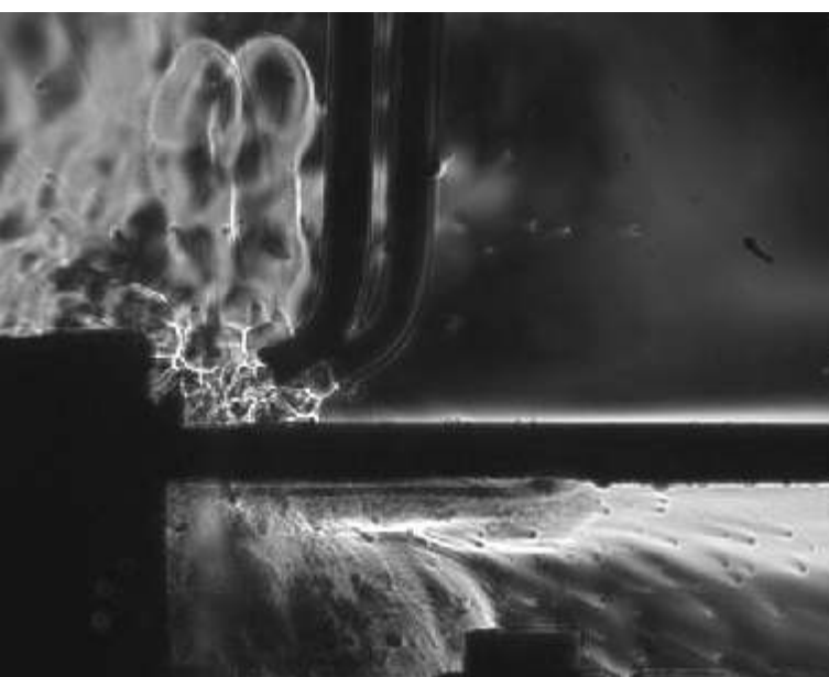
Schlieren image of a laser welding process
